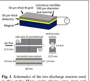
in this study: Micro cavity plasma array (top) and atmospheric pressure capillary jet source (bottom).
